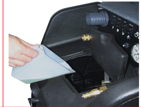
Add appropriate amount of chemical to water in solution tank
