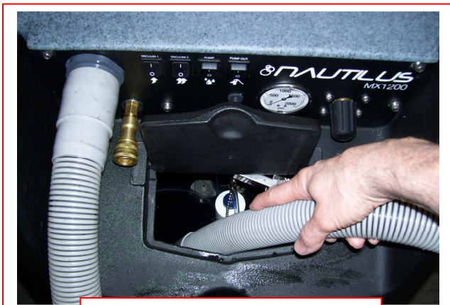
Vacuum water out of Solution Tank
